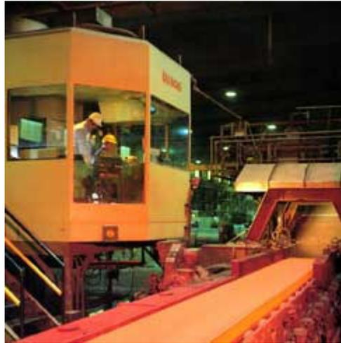
The cast bar is then reheated in a furnace and sent to the hot mill, where it is rolled and reduced in thickness.
